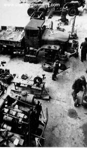
Left, 88th Maintenance Company's Automotive Maintenance Platon reconditions 5-ton trucks in open bays. Each of the squads work on two or three trucks at a time. Below, soldier uses a cutting forch to free a stuck too pintle. Below center, Below center, Below center, and Dana Howe spray paints a truck as one of the final steps. Bottom, Sp4 Gloria Maynard overhauls a sehtlich transmission.
